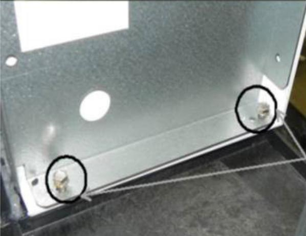
Remove 2) 1/4" screws where frame meets The base on the left hand side of the unit.
