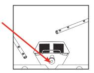
4. Wash tub must be completely filled before operating the wash pump to prevent damage to components. Once wash tub is filled, the machine is ready for operation.
