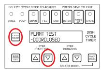
Press and hold the DRAIN button. The DRAIN output stays on while the button is held. The output turns off when the button is released. Repeat for the other seven buttons (use SAVE/EXIT to activate CYCLE output, use CYCLE COUNT to activate PUMP output). Second row of display shows outputs and inputs that are active.
