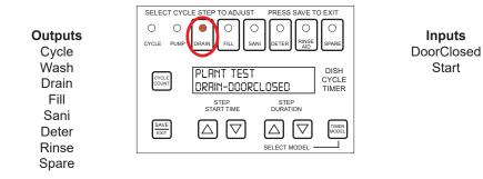
3. Plant test mode can also be used to prime chemicals if the machine has no priming function. Open door and press and hold the SANI button until sanitizer is seen entering the wash sump/tank and no air is in the line.
