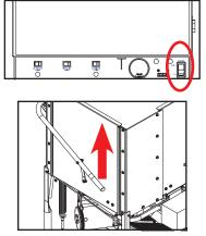
3. Remove drain stopper and allow tub to drain (WARNING! Wash tank water will be hot).
