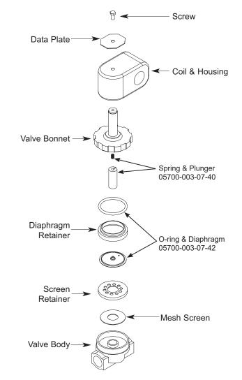
Complete 115 Volt Solenoid Valve Assembly 04810-100-53-00 Coil & Housing only 04810-200-01-18
