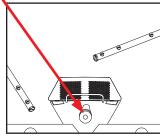
4. Remove sump strainer and pan strainer.
