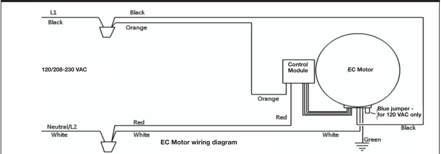
**NOTE:** EC motors have a soft start feature. When the power is turned on the control module gathers information from the motor then begins the start up process. After a few seconds the motor will start to turn and reach full set speed in 10-30 seconds.
