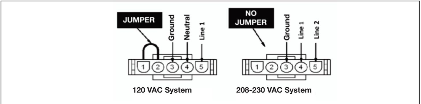
**CAUTION:** Operating the motor at 208-230VAC with the jumper will cause significant damage to the motor.
