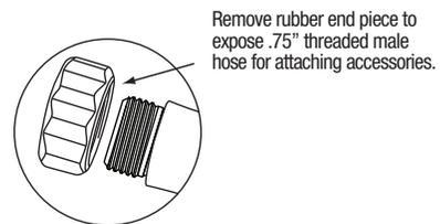
Remove rubber end piece to expose .75" threaded male hose for attaching accessories.
