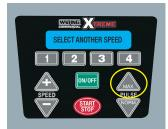
Press or button to set speed value. Set to 100%. Once desired speed is reached, press button to select speed. NOTE: Time starts at 5 seconds.
