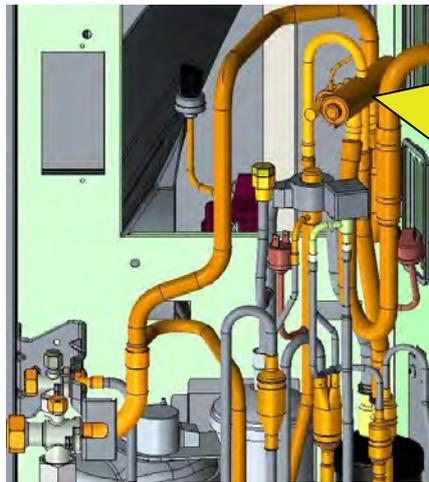
This is the position of the 4-way valve. Do not touch it directly with your hands. There is hot refrigerant at the exhaust pipe, so be careful not to be scalded.
