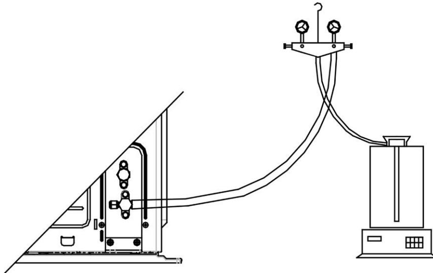
Step 5: Open the high pressure gauge valve (Keep the low pressure gauge valve closed). Then charge refrigerant into the system. Meanwhile, record the weight of refrigerant tank as m2.
