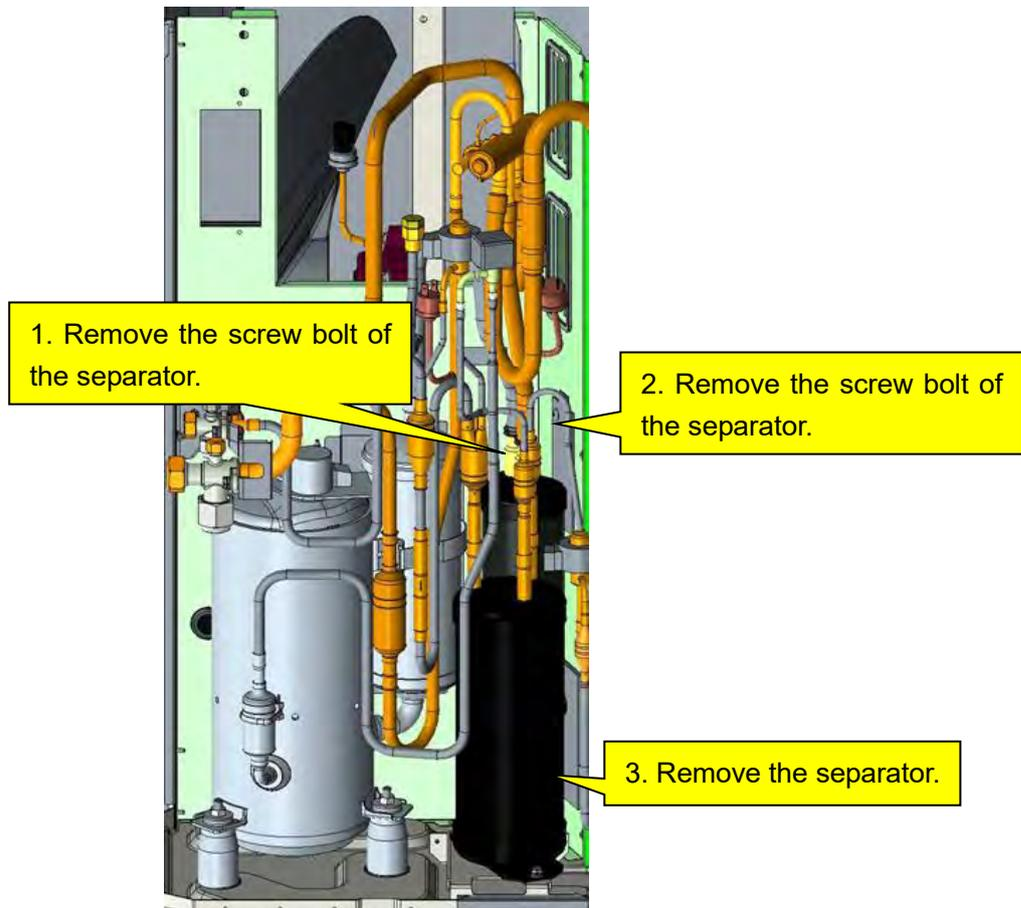
When the separator is detached, check whether there are impurities inside. Below is the checking method:
