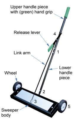
1. Connect the upper and lower handle sections by sliding the upper handle onto the lower handle. Align the (2) bolt holes in the upper and lower handles. Insert bolts with flat washers already on them through the bolt holes. Apply another washer and a lock nut to secure each bolt.
