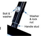
3. Attach one end of the link arm to the eye bolt on top of the sweeper body. Slide a washer onto a short bolt. Install the bolt through the bolt hole in the link arm. Put another washer on the end of the bolt; then insert it through the eye. Secure the bolt with another washer and a lock nut.
