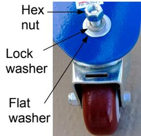
**Step 3:** Install the remaining caster and strap tab. Install a flat washer before connecting the yellow pull tab, and then install the TAB-BO, if you will use the nylon strap to pull the dolly, or TAB-TH, if you will use an optional rigid hook, followed by another flat washer, a lock washer and a nut. Tighten the nut against the lock washer.
