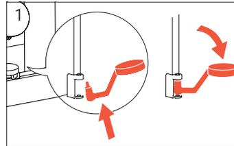
Insert cup support by tilting it into position.
