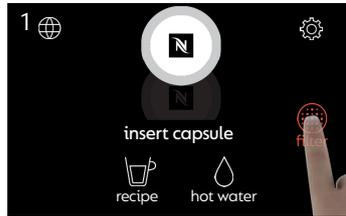
When the “filter” symbol appears in red the internal filter should be changed. Tap on red filter symbol and follow instructions on screen.
