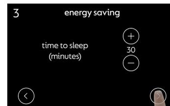
Select time after machine enters sleep mode. In this mode, a control panel has to be touched to turn on the machine again.
