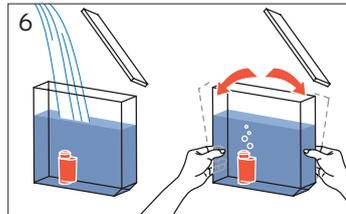
Fill water tank with fresh drinking water and attach lid again. Tilt the water tank back and forth to remove air bubbles from the filter.
