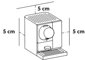
Please ensure the coffee machine is placed in a location with sufficient ventilation (at least 5 cm space on the back, on the sides and top of the machine).
