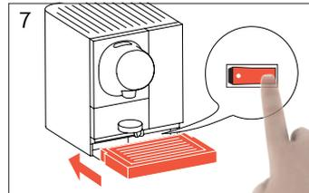
Switch on machine. Insert drip tray with drip grid.
