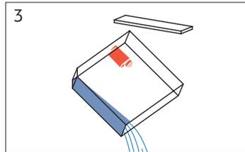
Remove water tank lid. Empty and rinse with fresh potable water.
