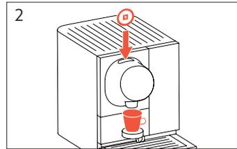
2 Place cup under the coffee outlet. Insert capsule into capsule slot.
