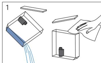
Remove water tank lid. Empty and rinse with fresh potable water. Dry with disposable tissue or paper towel. Attach lid again. Insert water tank back to machine.
