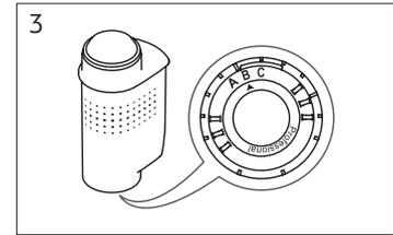
3 Adjust the bottom ring on the water filter to "A", "B" or "C" as recommended.
