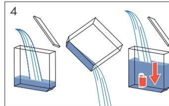
Remove water tank lid. Rinse with fresh potable water. Insert water filter into water tank. Fill water tank with fresh drinking water and attach lid again.
