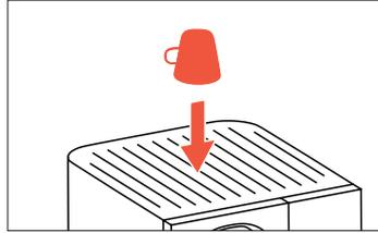
The cup heater is located on top of the machine. If a cup shall be heated, it must be placed upside down.
