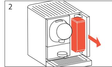
Remove water tank from machine. Clean tank.
