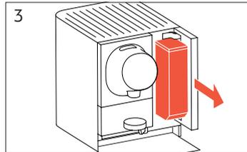
Remove water tank from machine.
