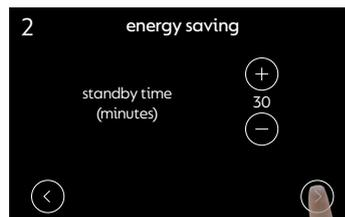
Select time after machine enters standby mode. In this mode, machine automatically turns on again if a user gets near the machine.
