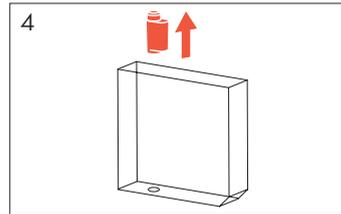
Remove old water filter from water tank.
