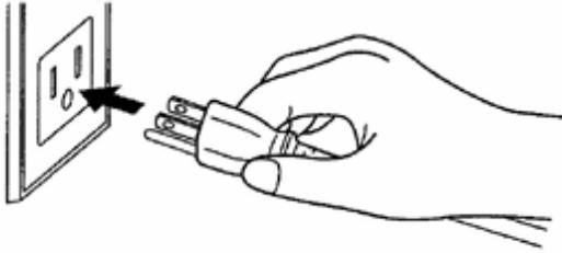
MAKING SURE THE ON/OFF SWITCH IS IN THE OFF POSITION, PLUG MACHINE INTO POWER OUTLET CHECKING THAT OUTLET IS OF THE CORRECT VOLTAGE.
