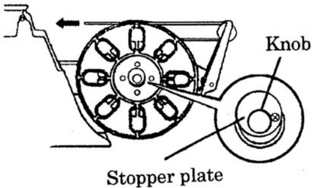
TO SECURE THE RIBBON SPOOL ONTO THE RIBBON SPOOL MANDREL SLIDE THE STOPPER PLATE UPWARD AS IN THE FIGURE TO THE LEFT, AND TIGHTEN THE KNOB SECURING THE SPOOL.
