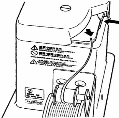
REMOVE THE TWIST TIE RIBBON FROM THE MACHINE BY PRESSING THE TIE HOLDING ARM AND PULLING BACK ON THE MATERIAL.
