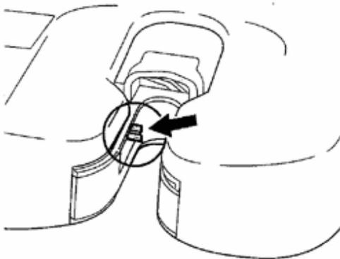
WHILE LOOKING INTO THE TYING APERTURE AND HOLDING THE TIE HOLDING ARM, CONTINUE PUSHING THE TWIST TIE RIBBON UNTIL IT APPEARS ABOUT 1/8" INTO THE TYING APERTURE. MACHINE IS NOW LOADED.
