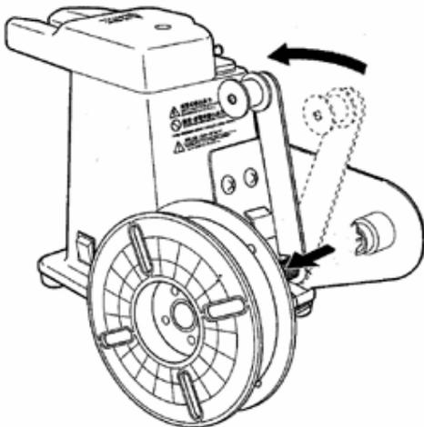
REMOVE THE ROLL OF TWIST TIE FROM THE RIBBON SPOOL MANDREL BY LOOSENING THE KNOB AND MOVING THE STOPPER PLATE TO THE CENTER OF THE TWIST TIE RIBBON SPOOL. TIGHTEN THE KNOB SO THE STOPPER PLATE IS EVEN WITH THE RIBBON SPOOL MANDREL. TO INSTALL A NEW SPOOL OF TWIST TIE RIBBON ON THE MACHINE FOLLOW INSTRUCTIONS IN SECTION 5.
