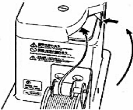
WHILE PRESSING THE TIE HOLDING ARM, INSERT THE TIP OF THE TWIST TIE RIBBON INTO THE MACHINE. **PLEASE NOTE IF USING POLYCORE NON-METALLIC TWIST TIE RIBBON ON THE MACHINE, WHEN FEEDING THE RIBBON IT IS IMPORTANT THAT THE CURL OF THE RIBBON GO IN THE DIRECTION SHOWN IN THE DIAGRAM TO THE LEFT. STANDARD TWIST TIES WITH METAL WIRE DO NOT HAVE A CURLING TENDENCY AND CAN BE FED IN ANY DIRECTION.**
