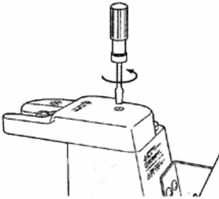
LOOSEN THE TOP COVER FIXING SCREW BY USING A SCREWDRIVER AND TURNING SCREW IN A COUNTER-CLOCKWISE DIRECTION.
