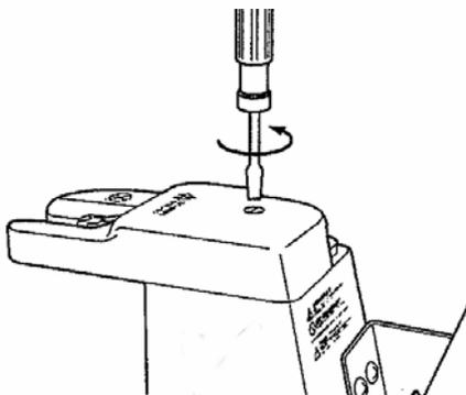
WHILE HOLDING THE TOP COVER IN PLACE, TIGHTEN THE TOP COVER FIXING SCREW.
