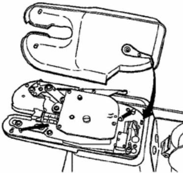
WHEN REPLACING COVER, PUT BACK ONTO THE TOP OF THE MACHINE SLOWLY MAKING SURE THAT THE PIN IS GOING INTO THE HOLE FOR THE SAFETY SWITCH. SEE FIGURE TO THE LEFT.
