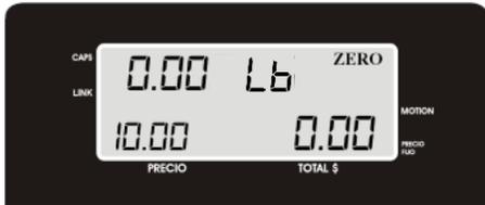
1.- Get the weight off the scale and use the numeric pad to type in the product's Price on the scale.
