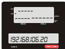
3.2.1.- By default the IP address is 192.168.106.20 with the arrow keys you can move around it's address and modify it.
