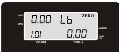
1.- Type in the PLU code in the scale, example 101, followed by the PLY key on the scale.
