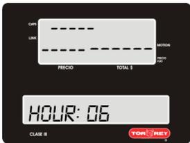
3.- Use the arrow keys to move around the digits and replace any of the digits with the number pad or press the DEL key or C key to erase a digit. Once you're done with the month press ENTER to go to minutes.
