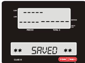
2.- Wait a few seconds while the scale configures this option and saves changes, once finished, it goes automatically into the sub-menu Configuration.
