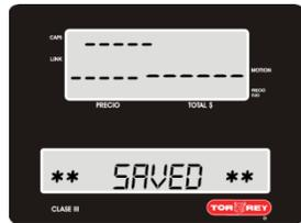
Once the parameters are saved, to be off the menu press the return key 4 times.
