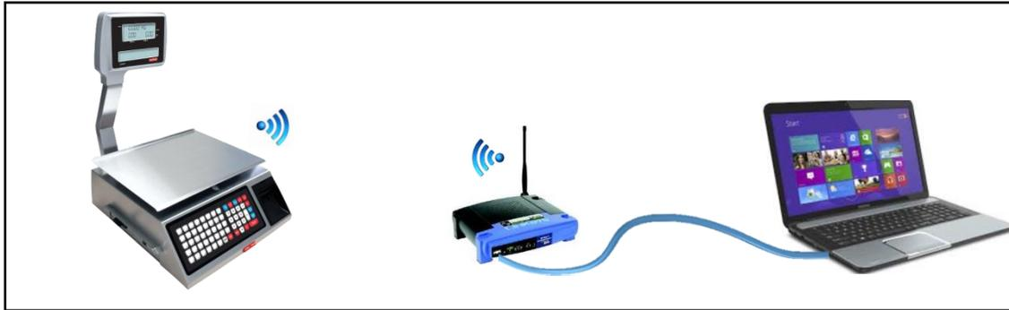
**The ETHERNET connection** is made with a network cable (RJ45) where you connect a modem, the scale and a computer
