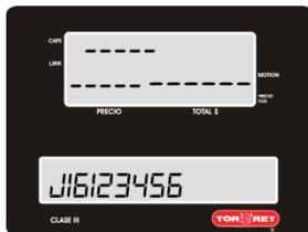
3.- When choosing SERIAL NUMBER the display will show the serial number on display and this number can't be altered by the user.
