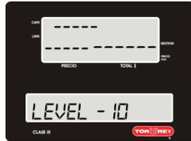
By default the intensity level is 7 the raise of level can slow down the printer.
