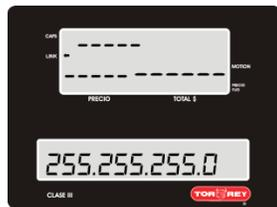
3.2.2.-By default the network mask is 255.255.255.0 using the arrow keys you can move around the digits, you will notice your current position due to the digit blinking when selected, you can replace the digit with a different one with the number pad. To erase a digit use the DEL key
