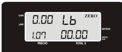
1.- Type in the product's codeo n the scale using the numeric pad followed by the **PLU** key on the scale.
