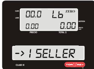
When selected the scale will go back to the main Screen and show the agent's name on the display for 3 seconds.
