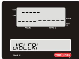
4.- -when choosing FIRMWARE VERSION the scale shows the version on display and this parameter its also incapable to be altered by the user.
