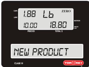
2.- Type in the Price of the new product and then place the product on the scale's plate, if you remove the weight off the scale the scale will go back to zero and the product's information would be gone.
