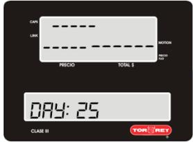
5.- Use the arrow keys to move around the digits and replace any of the digits with the number pad or press the DEL key or C key to erase a digit. Once you're done with the month press ENTER to save the parameters.
