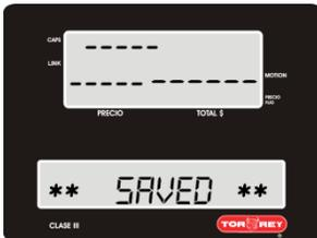
5.-When you save the changes, return to the OPERATION MODE menu, to exit and return to the normal functions of the scale only press the RETURN key 3 times .
