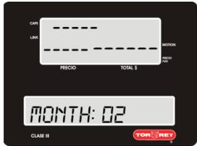
4.- Use the arrow keys to move around the digits and replace any of the digits with the number pad or press the DEL key or C key to erase a digit. Once you're done with the month press ENTER to go to DAY.
