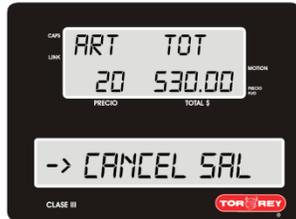
By using the arrows keys you can either choose the discount to apply or select to cancel the sale. On both cases press ENTER to finish the operation.
