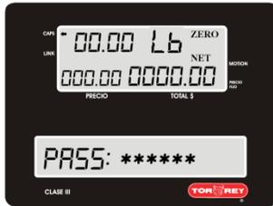
1.- Press the PROG button the word PASS will immediately appear in the advertising display: At this point, press the 123456 sequence and then press ENTER to enter the configuration menu.
