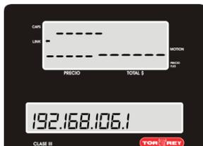
3.2.3.-.By default the gateway is 192.168.106.1 you can move around the digits using the arrow keys, you will notice your current position on the digits due to the certain digit blinkingyou can replace that digit using the numbers pad. To erase a digit use the DEL key or the C key, once finished editing press ENTER, then it will show the following messages:
