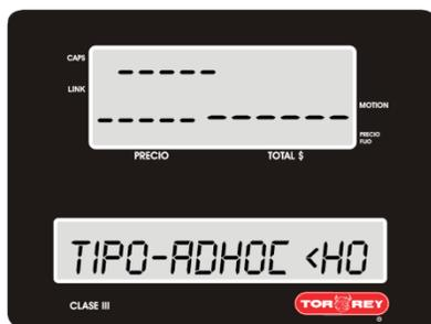
1.- Select the type of connection on the WLabel scale. ADHOC<HOT SPOT> Following section 13.2.3
