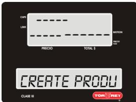
1.- To create a new product enter the CREATE PRODUCT option by following the steps in section 12 product configuration p.19 and then the sequence of this section.
