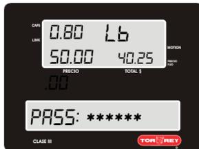
Immediately type in the password and press ENTER for the return to be applied.
