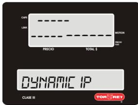
3.1.- When choosing DYNAMIC IP the scale configures automatically the necessary parameters for it to work dynamically on the scale.
