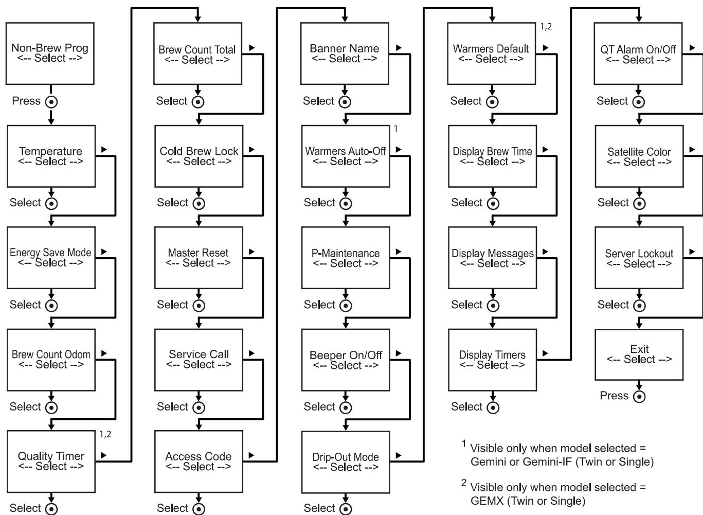
**Temperature** - sets the brewing temperature of the water held in the water tank. The factory default setting is 200°F/92°C (Gourmet STD). The setting range is 170°F to 206°F (77°C to 97°C). Once accessed, press **◀** or **▶** to choose the desired temperature. Then press **◎** to set and exit.
