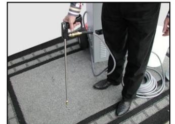
Note: keep vacuum hose out of the way while spraying Magnum Blue down. Next, disconnect spray gun and connect solution hose to floor wand, then connect vacuum hoses to both machine and floor wand.
