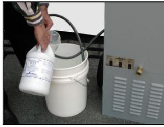
2. Connect 60 ft. Solution Hose to Scooter Machine, by pressing female quick connect all the way back, so that fully connect male to unit. Note: These two connectors must be all the way in for solution pump to run
