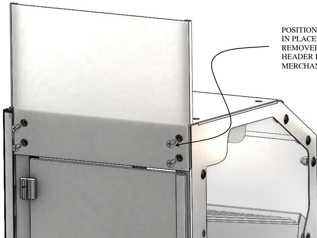
POSITION HEADER BRACKET IN PLACE. USING (4) SCREWS REMOVED IN STEP 1, ATTACH HEADER BRACKET TO MERCHANDISER.
