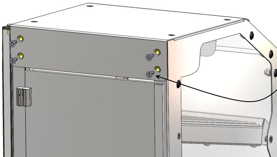
REMOVE (4) FLAT HEAD SCREWS FROM MERCHANDISER TOP AND SET ASIDE FOR USE IN STEP 2.
