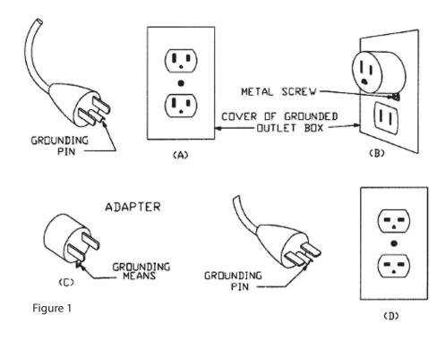
grounding instructions are not completely understood, or if in doubt as to whether the appliance is properly grounded. Do not modify the plug provided with the appliance – if it will not fit the outlet, have a proper outlet installed by a licensed electrician
