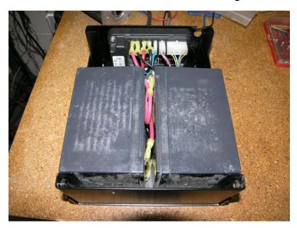
3. Replace battery box lid, and secure with 4 M6 screws.
