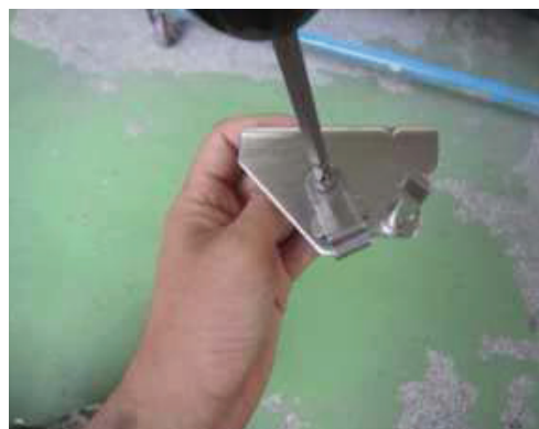
C-2. Disassemble bottom hinge (left).
