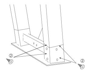
Place and secure Adjustable Footpad ① to bottom of the Table Base Legs (Part A).
