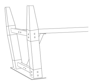
Secure Iron Side Bottom Braces (Part B) to Connector Bar (Part D) using Button Nut ③ from the outside and Button nut screw cap ⑤ from the opposite side using both Allen Wrenches simultaneously. Repeat for other side.
