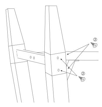
9 Then use Round cap Wire Screws ② to secure Iron Side Top Brace (Part C) from the sides.
