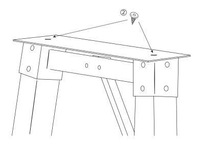
Place Table Top on top of Iron Side Top Braces (Part C).
