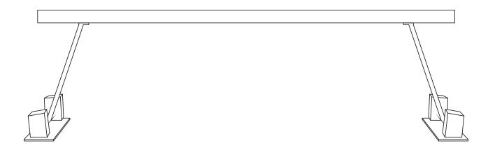
Secure them by using Combined Screw and 1 Flat Washer and 1 Locking Washer 4 from Brace Support (Part E) side. Repeat on opposite side.
