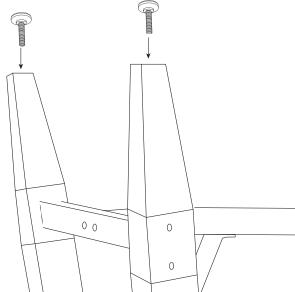
Next, turn base right side up. Secure legs to Iron Side Top Brace (Part C) using Round Cap Wire Screws ②.
