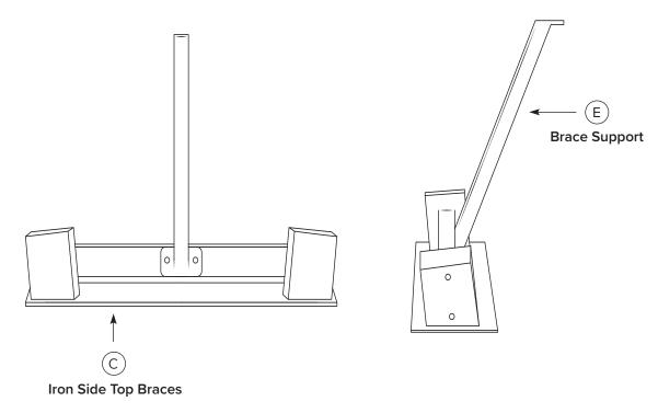
Secure both parts at pre-drilled holes using 2ea Button nut Screw Cap, ⑤ from the Brace Support (Part E), and 2ea Button nut ③ from the opposite side. Secure Button nut into Button nut Screw Cap using both Allen Wrenches simultaneously. Repeat for second pair.
