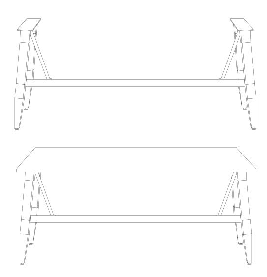
Secure by using Round Cap Wire Screws ② from underneath the top.
