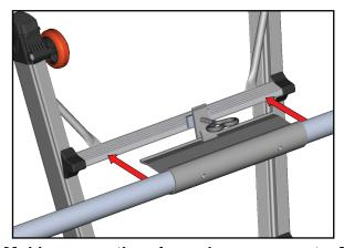
Making sure the clamp is swung out of the way, and the outer ladder assembly is extended at least one rung, slide the rung bracket onto the top outer rung.
