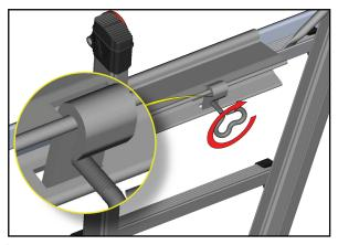
Swing the clamp around and hook it into the open slot in the rung bracket, then tighten the clamp onto the rung. If the clamp will not reach the slot, loosen the clamp all the way, and then try again.
