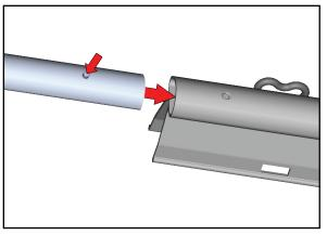
To assemble, hold down the spring pins and slide the arms into the rung bracket until the spring pins lock into place.
