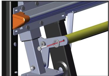
9. Insert the cap screw through the lock washer, angle arm and into the tube step. (As shown in the illustration).
