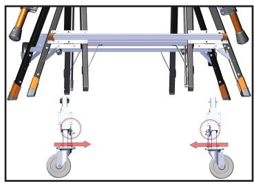
2. Make sure when you are lining up the two Wheel Lifts for installation that the two angle arms are facing towards each other. (As shown in the illustration).
