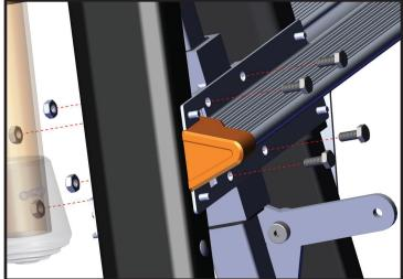
5. Insert 4 hex head screws into the bottom rung, through the Wheels Lifts and cap with lock nuts.
