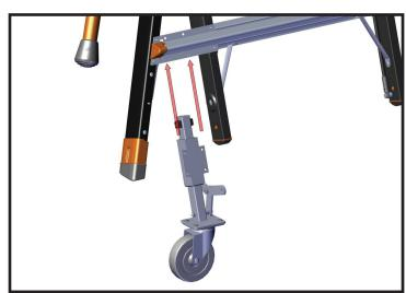
4. Insert the Wheel Lifts onto the bottom rung, and line up the holes.
