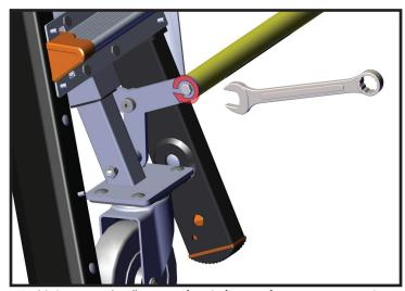
10. Using a 7/16" wrench, tighten the cap screw into place.
