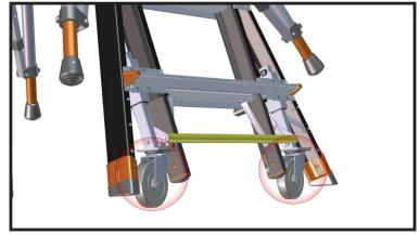
3. Once the Wheel Lift wheels are engaged, move to the other side of the ladder and repeat steps 1 and 2. The Cage will be able to move freely now.
