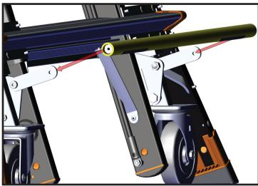
8. Line up the tube step and insert it making sure that it fits in-between the angle arms of the wheel lifts.
