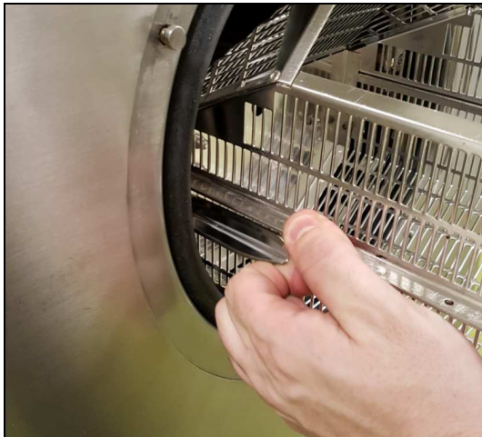
Figure 20 - Lock mechanism (the middle of the picture) which is pressed up to release the raw material basket; right and left side of the basket
