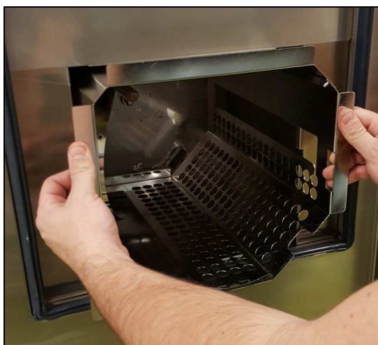
Figure 25 - Air duct plate pulled halfway out
