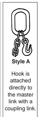
\*\*\* Cradle grab hooks standard; non-cradle hooks available on request. \*\* Style B slings are furnished with approximately one foot of chain. When using chain slings in a choke hitch, reduce the sling's rated capacity by 20%.
