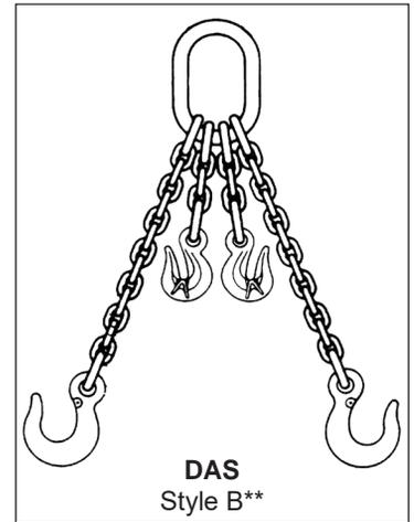
\*\*\* Cradle grab hooks standard; non-cradle hooks available on request. \*\* Style B slings are furnished with approximately one foot of chain. When using chain slings in a choke hitch, reduce the sling's rated capacity by 20%.
