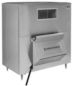
Seal the entire interior and exterior perimeter of the snout with silicone sealant to prevent water leakage
