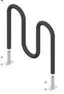
Slide Main tube (Item #1) over two foot plates (Item #2) and secure foot plates to main tube using supplied 5/16-18 hardware (Item #3) in (4x) places.
