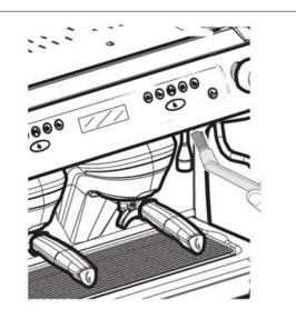
Use the supplied bush to clean the hole where the hot water nozzle is located.
