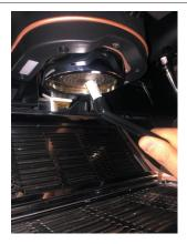
Use the supplied brush to clean the perforated disk's position.
