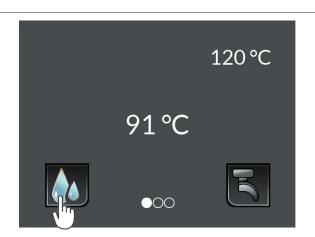
Before dispensing, press the purge button to wash the espresso dispensing unit's perforated disk.
