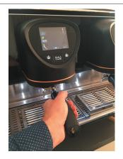
Insert the filter holder into the unit to be washed.
