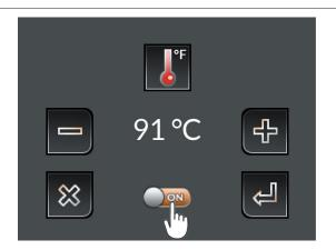
Use the +/- buttons to set the desired temperature and turn the activation selector to its ON position.
