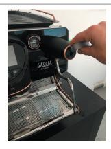
Push the steam lever upwards and hold it in that position for several seconds; the lever will return to its original position once released.
