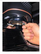
Use an appropriate tool to leverage the perforated disk, taking care not to damage the unit's gasket.
