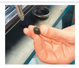
Pass a pipe cleaner through all the nozzle's holes to eliminate any residues.
