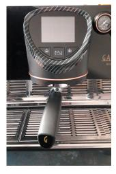
Fill the filter holder with ground coffee, compress it, and insert it into the espresso dispensing unit.
