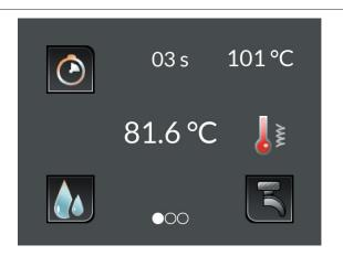
The elapsed time is displayed as long as the dispensing operation is in progress.
