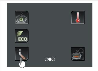
Press the indicated button to start the wash cycle.
