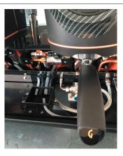
The wash water is discharged into the tray through the espresso unit's solenoid valve.
