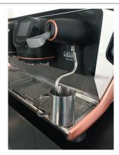
Immerse the steam nozzle in the receptacle containing the beverage to be heated and press down, or else press and hold the steam control lever in the upward position.
