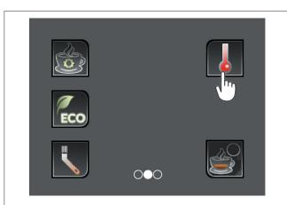
Press the indicated button to access the espresso boilers' activation screen.
