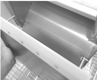
The #2 scraper lays on top of the bottom roll and is attached to the discharge tray as one piece. To remove the tray reach under the discharge tray and detach the scraper springs from the pins. Lift the tray up towards the machine and scraper will dislodge from the scraper pins.
