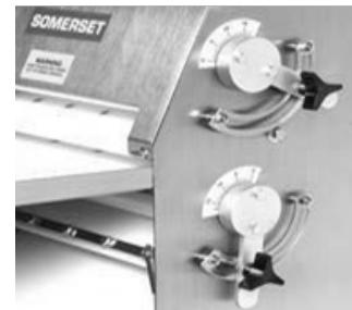
**The bottom roll dial is Aligned with the number “2”**
