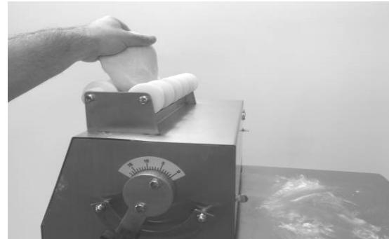
**\*\* If dough does not slide easily on the discharge trays, dust the trays with flour. \*\***
