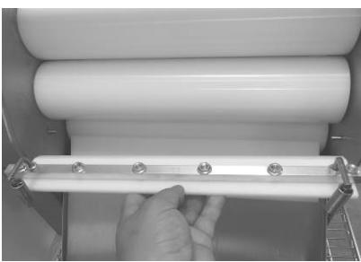
The #1 scraper lays under the middle roll and attaches to the scraper pins on the inside walls of the machine. The beveled edge points in between the middle and bottom roll.
