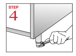
Level dishmachine by adjusting leveling legs. Dishmachine must be level, front and back, to ensure proper performance.
