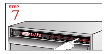
Hold down "FILL" Switch for approximately 10 - 15 seconds to allow water to flow into the dishwasher. The 4th cam of timer assembly has to be adjusted to maintain the same water level during the cycle.
