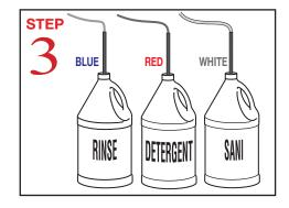
Insert tube stiffener with chemical tubing into each corresponding chemical dispenser.
