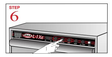
Press and Hold down "SANI", "DETERGENT" and "RINSE" switches to prime chemicals. This step must be repeated each time chemical containers are changed.
