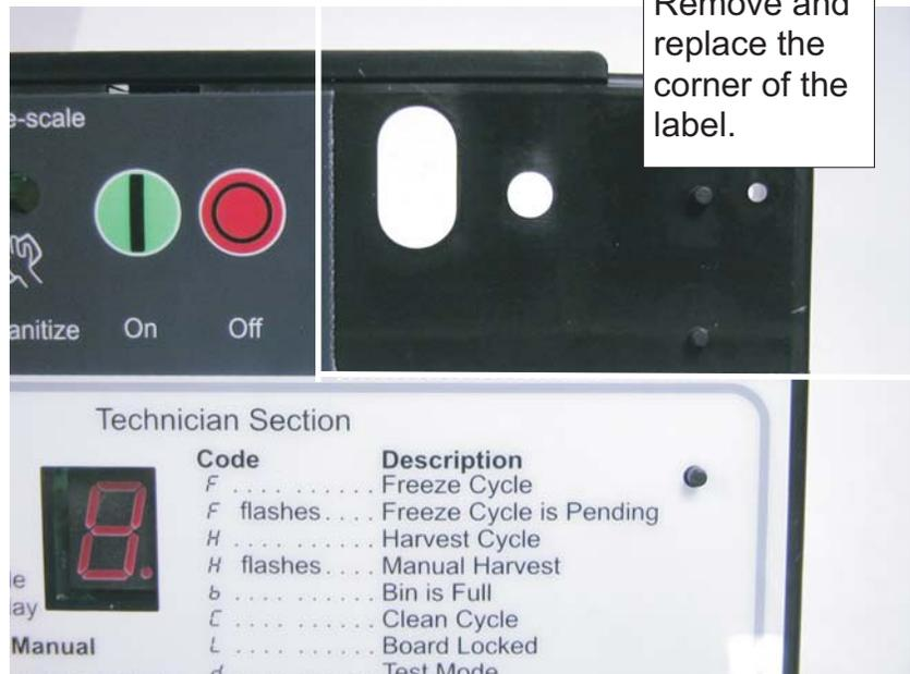
5. Attach supplied label to control box door in place of the section removed in step 4.
