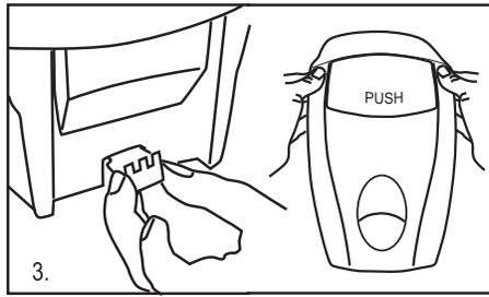
3. Re-install the latch piece in the bottom of the dispenser with the SLOTTED SIDE AWAY from the wall and toward the front of the dispenser. Push the latch piece into the dispenser until it snaps into place.
