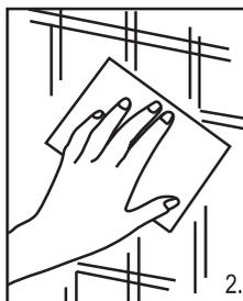
2. Clean the mounting surface thoroughly using any type of general purpose cleaner and a paper towel. BE CERTAIN THE SURFACE IS COMPLETELY DRY BEFORE PROCEEDING.
