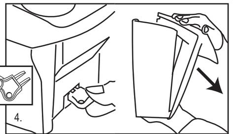
4. To OPEN, insert the key into the slots of the release latch on the bottom of the dispenser and push the key up. Place your other hand on top of the dispenser and guide the front cover forward.
