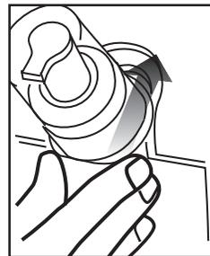
3. Slide the bag collar over the guide and push. Be certain the bag collar is completely inserted in the collar guide.
