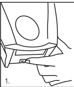
1. Open the dispenser by pushing up on the release latch (or with the key if you have converted to the keyed locking mode). The latch is on the bottom back edge of the dispenser in the center. While pushing the release latch, open the dispenser by placing your other hand on the TOP, and guiding the front cover forward.
