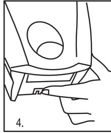
4. Open the dispenser by pushing up on the release latch. The latch is on the bottom back edge of the dispenser in the center. NOTE: See "Keyed Locking Option" if you wish to convert your dispenser to keyed system.
