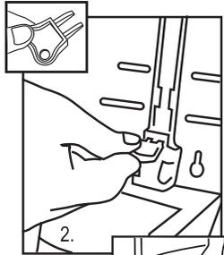
2. From INSIDE the dispenser, insert the key into the back of the dispenser in the key slot and push until the latch piece is ejected from the bottom of the dispenser.
