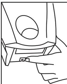
3. Open the dispenser by pushing up on the release latch. The latch is on the bottom back edge of the dispenser in the center. NOTE: See "Keyed Locking Option" if you wish to convert your dispenser to keyed system.
