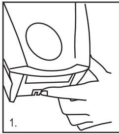
1. Open the dispenser by pushing up on the release latch. The latch is on the bottom back edge of the dispenser in the center. While pushing the release latch, open the dispenser by placing your other hand on the top and guiding the front cover forward.
