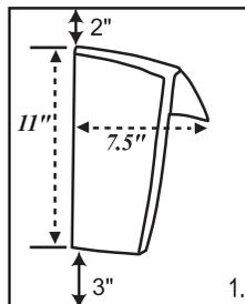
1. **IMPORTANT:** Dispenser opens to the front. For ideal placement, the dispenser should be mounted 3" above any countertop, fixture or obstruction and 2" below any upper cabinet, fixture or obstruction.
