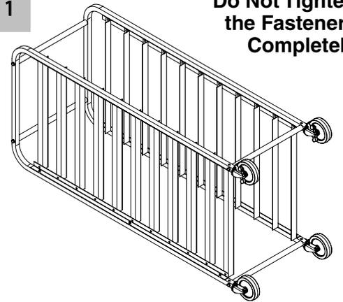
Do Not Tighten the Fasteners Completely
