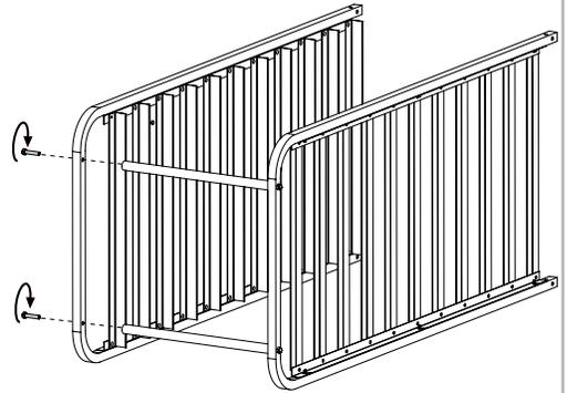
6 Do Not Tighten the Fasteners Completely
