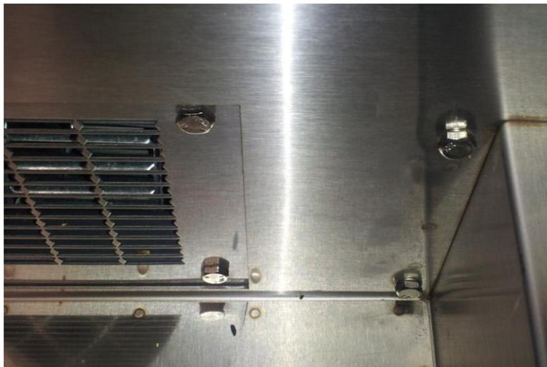
Position the blower box on the outside of the table with the blower mounting bolts (as shown above) so they fit inside the two cut outs on the inside of the table. Then use the four 1/4-20x1/2 bolts and lock washers inside of the bin, through the table wall into the weld nuts inside of the box.
