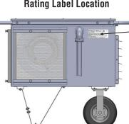
MODEL:PCKW2030-3 VOLTS:208 50/60 Hz PHASE:3 WATTS:25 KW AMPS:74.9
