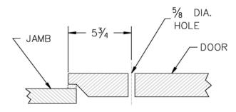
**1.** Drill hole for plunger rod of inside release handle. The hole, 5/8" (15.87mm), is drilled 5-3/4" (136.05mm) center distance from edge of door as shown in illustration.
