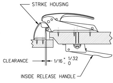
**5.** Attach inside release handle. (Three No. 12 (5.5mm) screws are required.) **NOTE:** The inside release handle can be mounted for use in a horizontal, up or down position.
