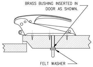
**4.** Insert brass bushing and felt washer. Slip the brass bushing onto the plunger rod. Push the bushing flush with the door (as shown in the illustration). Slip the felt washer onto the plunger rod, flush against the brass bushing.
