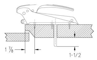
**3. Fasten latch to door.** Six No. 14 (6mm) screws are required. **IMPORTANT!** The front screw-hole must be located on a 1-7/8" (47.63mm) center from edge of door as shown in illustration.
