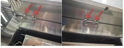
Scrape open the glass glue on the left and right sides of the top board with a blade. If there is no blade, insert other thin blades into the gaps of the top board and cut along the red line direction. After completion, the top board can be removed.
