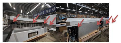
Remove the screws from the top board supplement: To remove the screws from the front of the top board, you need to remove the upper drawer and control panel separately to remove the screws. For the upper drawer, you need to release the red buckles on both sides upwards and lift them up when pulling them out to remove the drawer, the below image is for your information.
