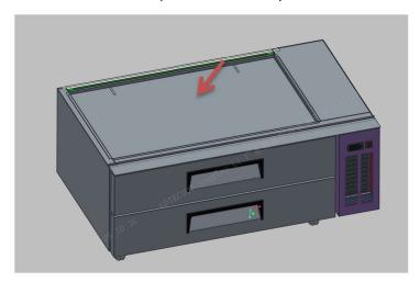
IV After removing it, you can see the evaporator cover. Remove the screws of the evaporator cover and take it out.
