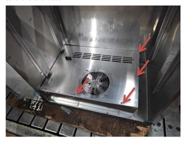
V Remove the fan motor that needs to be replaced (loosen the installation screws under the fan motor and unplug the fan wiring terminals from the wiring harness). If the fan blades are not ready, they can be removed and replaced on the new fan motor.
