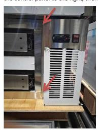
After removing the drawers and control panel separately, you can remove the screws at the front of the top board. There are 4-5 connection blocks on the top board, and dismantling the top board only requires removing the 2 screws connecting each connection block to the top board.
