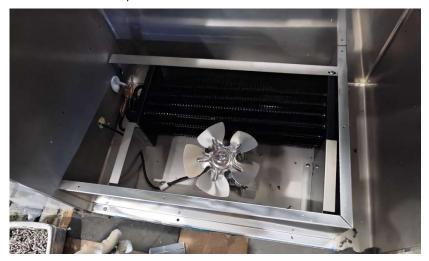
VII Reinstall the evaporator cover. After installing the evaporator cover, it is best to use iron wire or other slender tools to rotate the fan blades through the fan motor cover and check if they are stuck.
