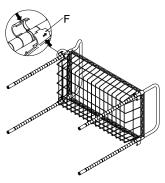
Snap two slip sleeves into the top groove of each pole with the arrows facing up. If necessary, move the sleeves slightly up or down until it "snaps" into place
