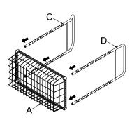
Insert the pole of left & right panel to the collar of the top of the bottom basket
