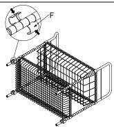
Snap two slip sleeves into the last 2nd bottom groove of each pole with the arrows facing up. If necessary, move the sleeves slightly up or down until it "snaps" into place 6
