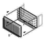
Insert the pole of left & right panel to the collar of the bottom basket
