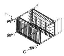
Screw caster stem completely into each bottom of post. **Tighten securely**. Make sure that the locking casters are on the same side.
