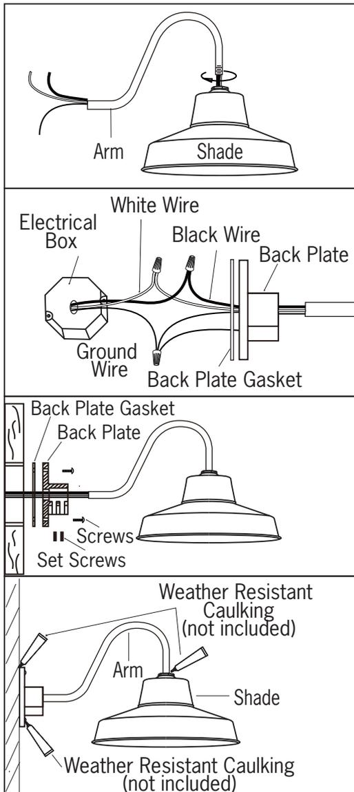
**WARNING: SUITABLE FOR WET LOCATIONS WHEN THREADS ARE SEALED WITH TEFLON TAPE OR PIPE SEAL.**
