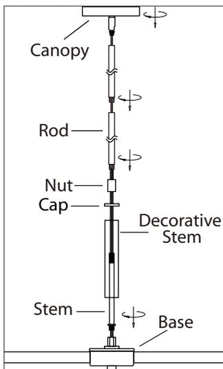
**1.** Install the stem onto the base. Slide the decorative stem onto the screw stud. Tighten the cap against the assembly by the nut.
