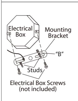
**3.** Loosen "B". Adjust stud to desired length and lock in place with "B". Mount the mounting bracket to electrical box using electrical box screws (not included). Make sure the studs on the mounting bracket are facing out from the electrical box.
