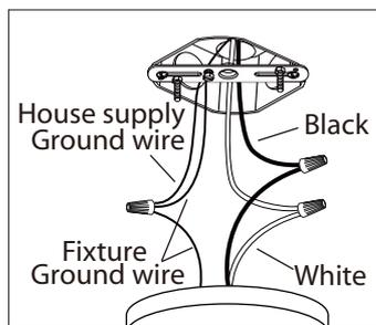
**4.** Connect the ground wires (bare copper or green) from your fixture to the ground wire (bare copper or green) or ground screw in the electrical box. Connect the black wire (or wire with marking) from the fixture to the black wire in the electrical box and connect the white wire from the fixture to the white wire in the electrical box.
