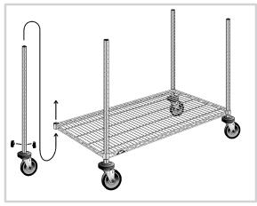
2. Install the remaining two shelves as shown and seat each corner with a mallet or a hammer and board.
