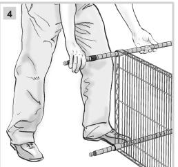
Stand the 18" x 60" wire shelf on its side and, working from the bottomside of the shelf, slide the four posts up through the post holes until the plastic sleeves on the posts are seated. Note: the mat wires are on the top of the wire shelf and the collars are thicker at the bottom.
