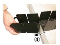
1. The EcoTrac Spring Glide has a series of break away sections. (<u>NOTE</u>: Wear EYE PROTECTION before proceeding.) To shorten a glide, line up break away point of sections to be removed over the edge of a table, then push down to snap the outer walls. Twist the free section in order to remove.
