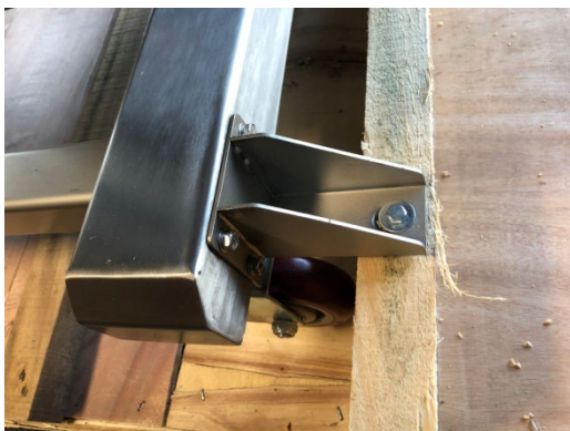
Figure 6. Bolts locking HL-M1120LD to crate.
