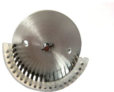
Figure 18. Ensure two holes and pins line up with the base
