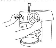
5) By holding the upper end of main shaft, turn the ice block holder at the other end of the shaft counter-clockwise and remove it from the main shaft.
