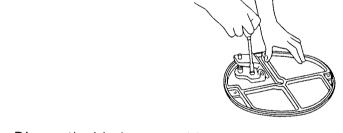
• Dismantle blade assembly-consisting of base plate, stopper ring, spring, blade fitting plate and blade fitting plate shaft.
