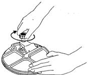
• Unscrew the (2) screws fastening blade assembly to shaving plate and remove blade assembly.
