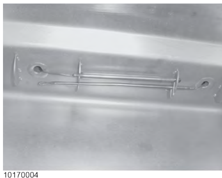
Figure 2-2 Thermostat Sensing Bulb - Gas
