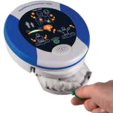
12. Tear open the pouch to remove the electrode pads.
