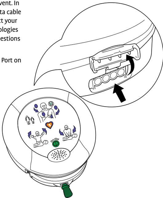
2. Connect the USB connector on the data cable to a PC.
