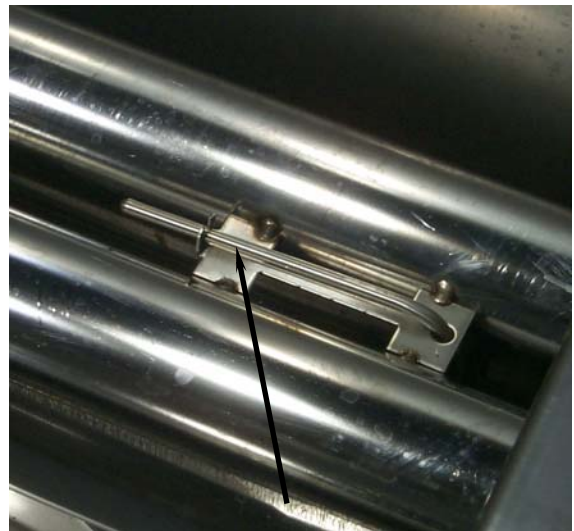
Electronic thermostat probe in frypot (arrow).
