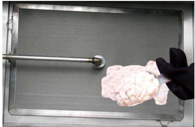
Applying filter powder to filter-leaf.
