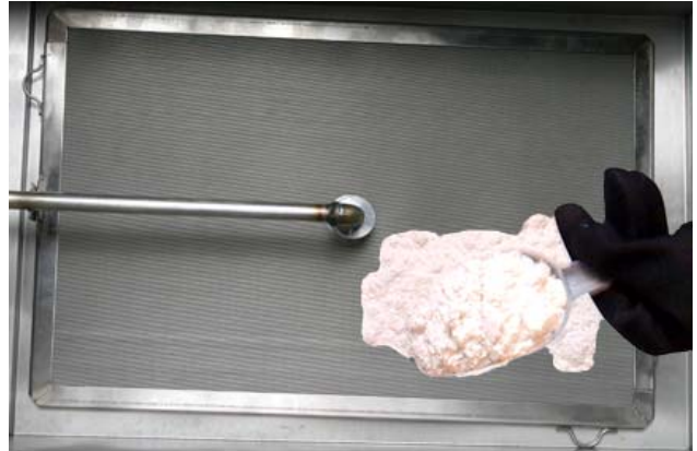
Applying filter powder to filter-leaf.
