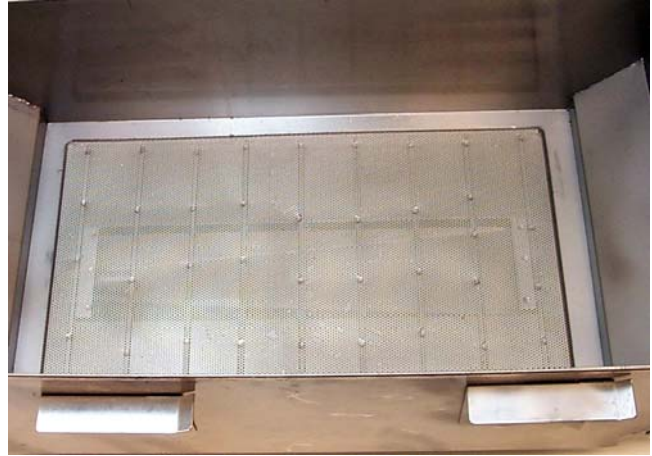
Support grid properly placed in filter pan.
