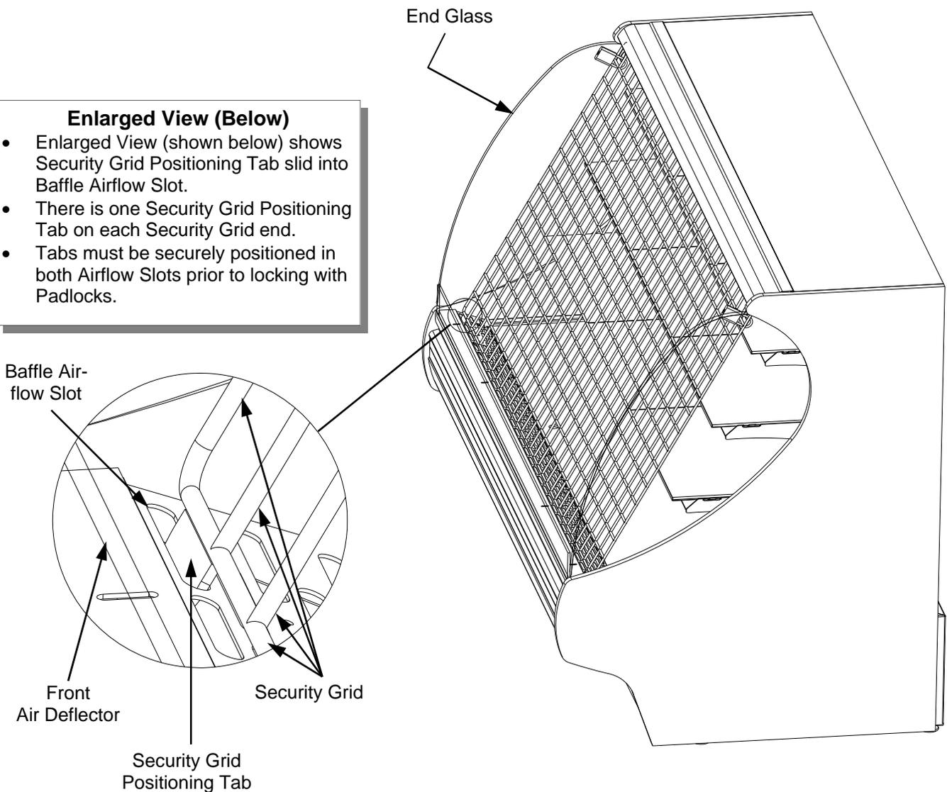
**2. Securing Security Grid Into Place and Locking**
