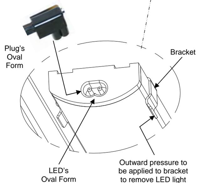
**5. Proper Plug Insertion Into LED Light**
