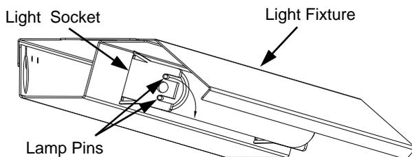
Above Photo Illustration shows Light Fixture. To remove lamp, simply rotate lamp clockwise and out. To replace, place one set of pins into slots and rotate second set of pins into slots.
