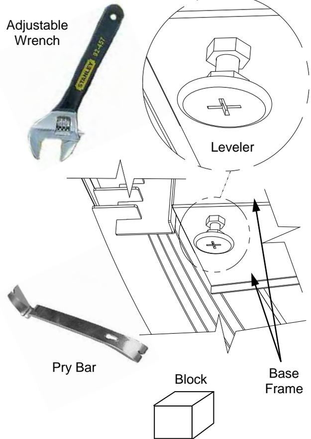
**3. Frame Support Rails Must Be Shimmed**
