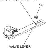
Insert the black snap bushing, (Item 13) into 3/8" (10mm) diam. hole of valve lever. Valve lever is attached to water regulator and push button located at top of cooler (not shown).
