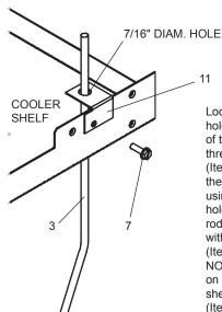
Locate the 1" (25mm) diam. hole in the right front corner of the cooler shelf. Insert the threaded end of the push rod, (Item 3) through this hole. Place the alignment bracket, (Item 11) using the 7/16" (17 mm) diam. hole over the end of the push rod and secure to cooler shelf with (1) #10 x 5/8" long screw (Item 7).
