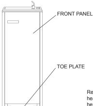
Remove toe plate (2, phillips head screws) and front panel (2, hex head screws) from cooler.
