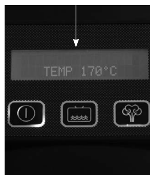
The machine needs about 8-10 minutes to convert the water into dry vapor. Once it reaches operating pressure, this appears on the display (4).and the display signals that it is ready for use.
