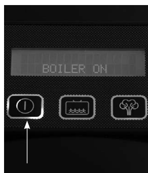
Switch on the unit by pressing the main switch (3) Now the boiler is turned on and the machine will pump water into the boiler.
