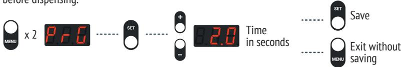
**Calibration** is needed if the displayed volume does not correspond with the actual volume dispensed.
