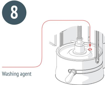
Wash flask drainage line by pumping washing liquid appropriate to the a treatment stage through current it.
